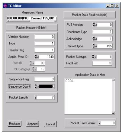
Double clicking on the Application Data box allows you to edit the first 4 words of the parameter in decimal. The Packet error control and source seq. controls are automatically updated during execution.
